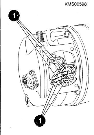
Unscrew ribbon cable (1) from contact rail (2) of starting-motor solenoid to term. 30.
